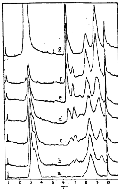
Fig. III.5.4 NMR spectra of solutions of methyl methacrylate-styrene copolymers and homopolymers, 0.10 g. in 0.5 ml. of \text{CHCl}_3 or \text{CCl}_4 , (see text) with 2% tetramethylsilane as internal reference ( r = 10.00 ): (a) polystyrene; (b) 10:90 (methyl methacrylate-styrene mole ratio in monomer feed); (c) 25:75; (d) 50:50; (e) 75:25; (f) 90:10; (g) polymethyl methacrylate.
