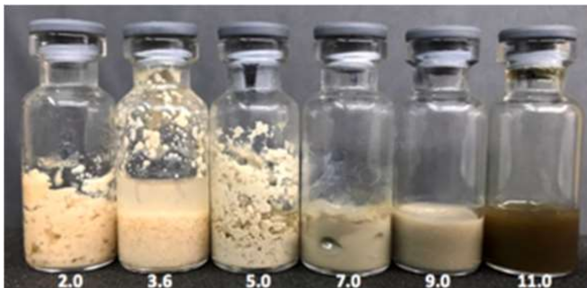
fig. 5. Gels formed from huauzontle protein isolates dispersions (15 g/100 mL) at different pH values.
