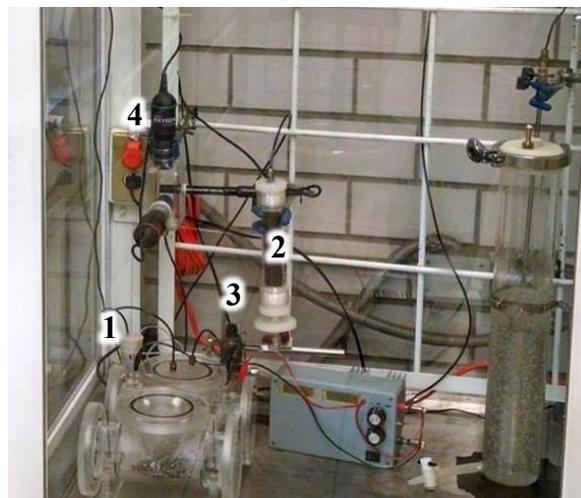
Figure 2. Respirometer for solid state culture analysis. Humidifier on the inlet to the bioreactor (1), drier column on the outlet of the bioreactor (2), flow meter (3) and sensor chamber to measure CO<sub>2</sub> and O<sub>2</sub> concentrations and relative humidity in the air flow (4).
