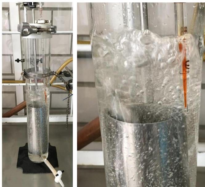
Figure 1. Experimental arrangement for interfacial hydrocarbon mass transfer quantification, pipet contains rhodophile stained hydrocarbon blend.
