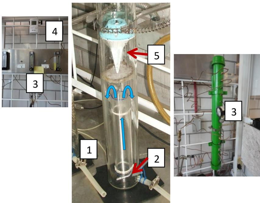
Figure 1. Airlift bioreactor arrangement. Image shows the bioreactor body (1), gas diffuser (2), pressure and gas flowrate control (3), temperature control (4) and foam breaker (5).
